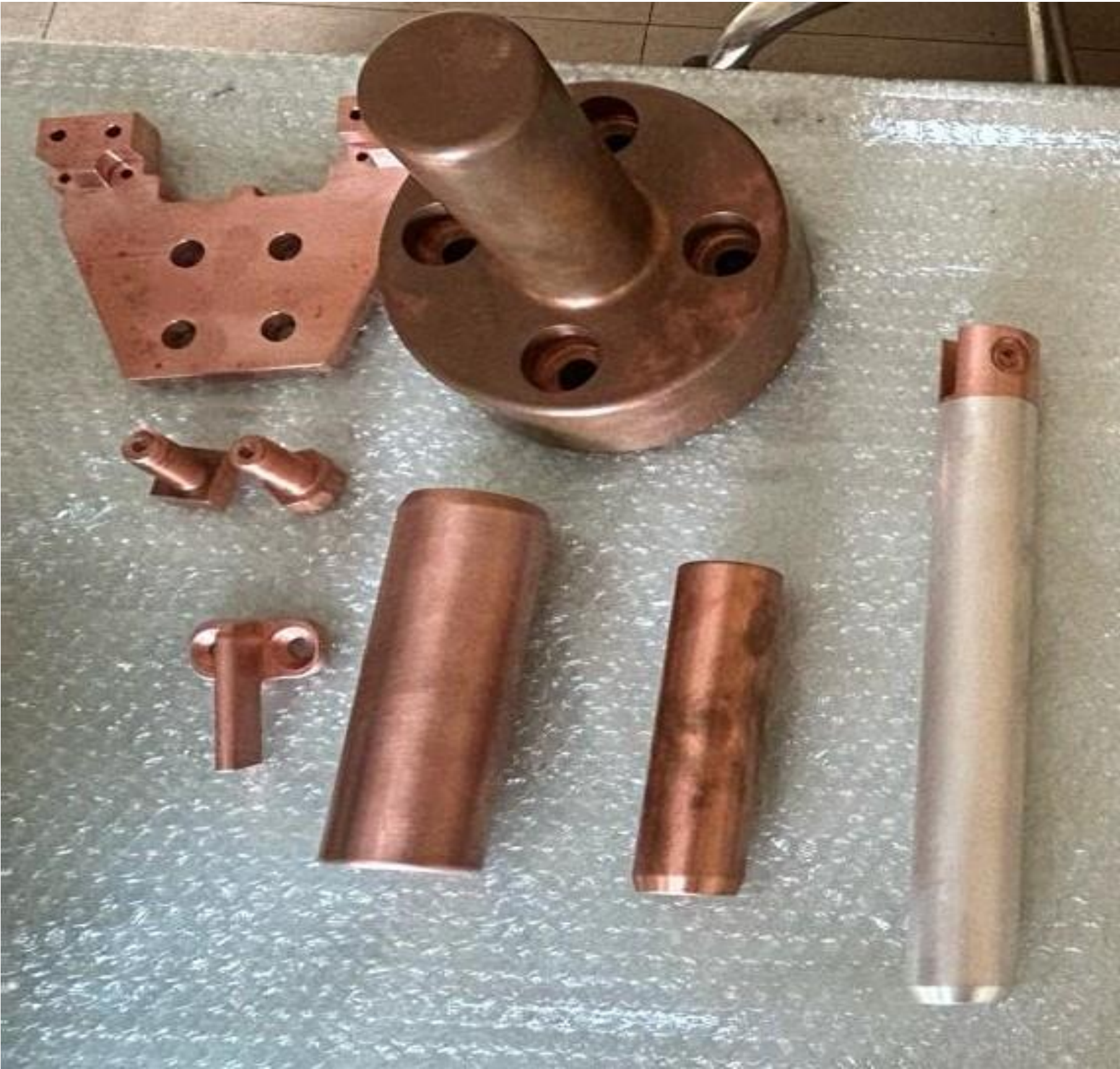
Switchgear Machined Copper Components
